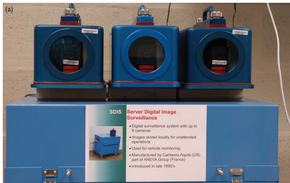
FIG. 23. IAEA monitoring and safeguard facilities: (a) video cameras used for remote monitoring of nuclear sites; and (b) the IAEA Safeguards Analytical Laboratory.
